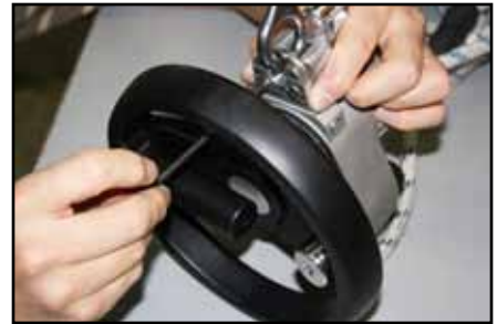
Step 3 - While holding the adapter and plate in place, insert the two screws and tighten until snug.
