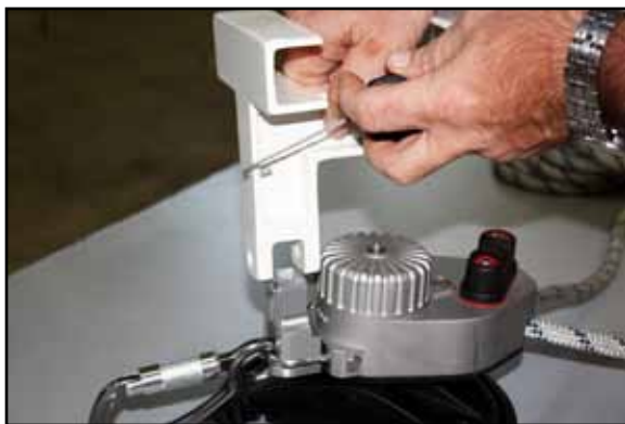
Step 4 - Place the ladder bracket onto the adapter assembly.
