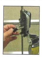
A)Release pull pins by depressing end buttons and remove from unit
