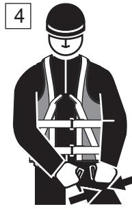
Fasten the thigh straps putting around each strap around the thigh. The straps mustn't be twisted. Adjust the straps. The harness should be tighten but not uncomfortable.
