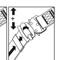
Connect the elements of the buckle to hear "click" sound. Verify if the buckle is blocked and working correct.
