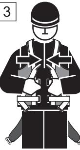
Connect the belt and shoulder webbing buckles. Adjust the straps so the harness fits the body, not too tight. It is forbidden to use the harness with disconnected buckles.
