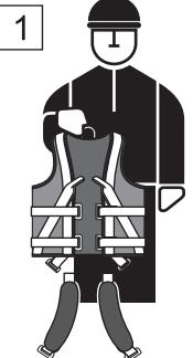
Hold the harness by dorsal D-ring. The straps should be unfastened and free.
