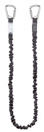
Antistatic, flame retardant energy absorbing lanyard with rescue ring, acc. To EN 354 and EN 355. Made of 35 mm wide antistatic-conductive Aramide tubular webbing. Energy absorber with very gentle tear behavior. Stainless steel hook with TRI-lock closing. Length max. 2 m.
