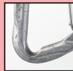
Significant material abrasion  $\geq 20\%$
